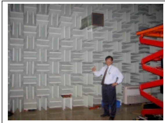
Figure 6 - Daikin Applied's Anechoic Test Facility
