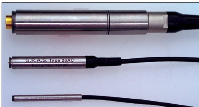
Figure 3. G.R.A.S. 1/2-inch, 1/4-inch and 1/8-inch microphone preamplifiers based on semiconductors and ceramic substrates.
