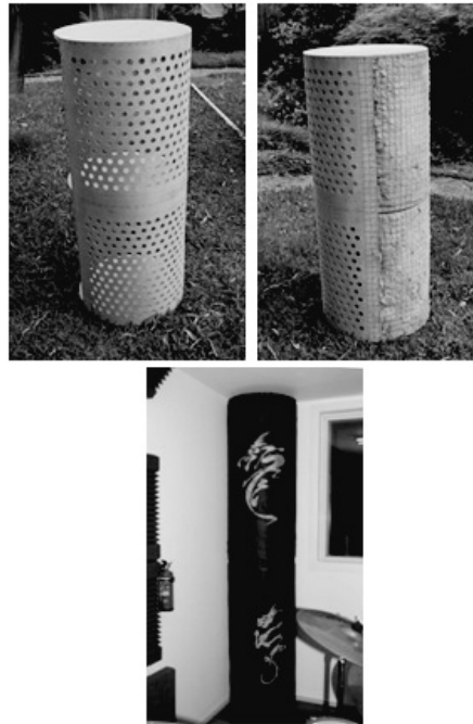
Figure 11. Construction Details of Tube Traps; Plywood Frame (upper left); With Rockwool Infill (upper right); Corner Installation in Studio (bottom)
